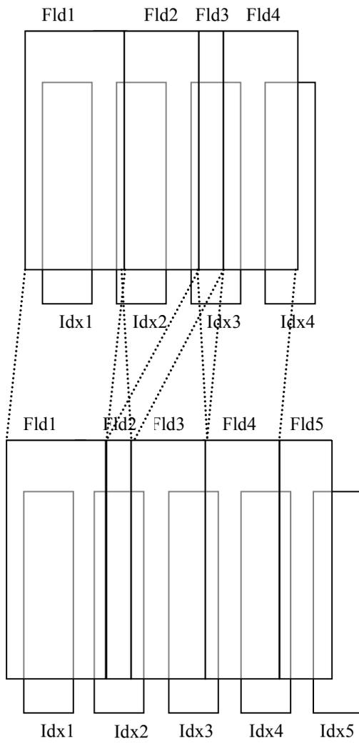
Figure 7. Concatenating two UBFiles together to form a new UBFile.
