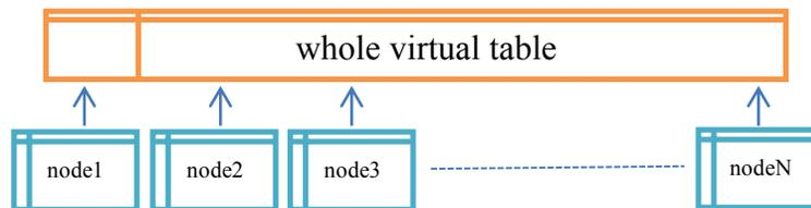
**Figure 9.** A whole table is a virtual table representing a union of node-component tables visible on the nodes.
