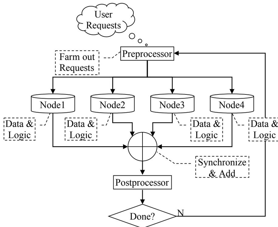
Figure 2. UBX™: user requests execute simultaneously on multiple nodes.
