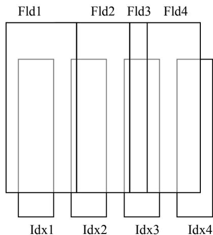
Figure 5. The basic UBFile structure: fixed format data with all fields indexed and stored individually.
