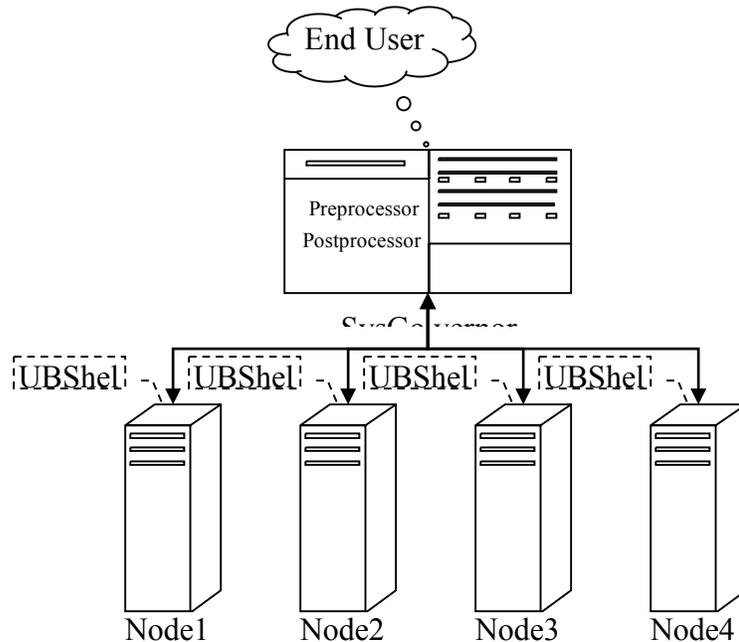
Figure 3. Physical View of UBXTM: SysGovernor and nodes are networked together.
